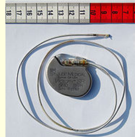
Artificial pacemaker with electrode for transvenous insertion.
