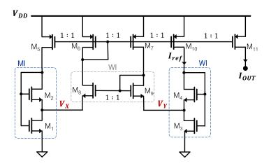
Figure 16. Self-biased current source (SBCS) circuit.
