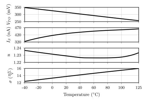
**Figure 7.** Parameters of the 4PM vs. temperature of a medium (nominal)  $V_T$  NMOS transistor with  $W/L = 1 \ \mu m/0.3 \ \mu m$ .
