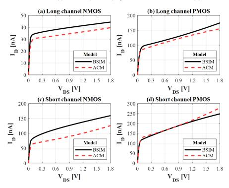
**Figure 9.**  $I_D \times V_{DS} \otimes V_{GS} = 200 \text{ mV}$  for (**a**) medium (nominal)  $V_T$  long-channel NMOS and (**b**) PMOS transistors and for (**c**) medium (nominal)  $V_T$  short-channel NMOS and (**d**) PMOS transistors.
