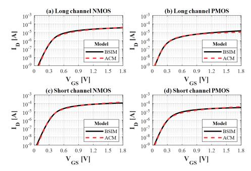
**Figure 8.**  $I_D \times V_{GS} @ V_{DS} = 200 \text{ mV}$  for (**a**) medium (nominal)  $V_T$  long-channel NMOS and (**b**) PMOS transistors and for (**c**) medium (nominal)  $V_T$  short-channel NMOS and (**d**) PMOS transistors.
