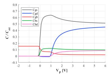
**Figure 4.** Capacitances (15)–(19) normalized to  $C_{ox}$  versus the pinch-off voltage for  $V_{DS} = 1$  V.
