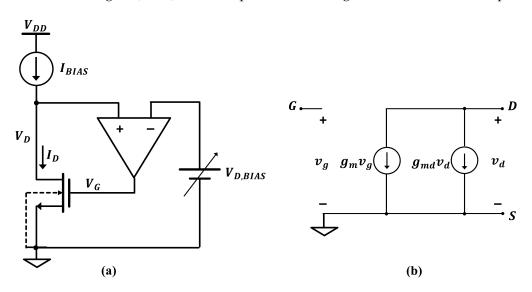
Figure 6. (a) Circuit to determine the CSIG and (b) its equivalent small-signal model.
