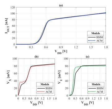
**Figure 17.** Results of DC analysis for voltage sweep on  $V_{DD}$ : (a) output current, (b)  $V_X$  and (c)  $V_Y$ .
