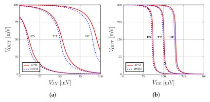
**Figure 12.** Voltage-transfer characteristics of the CMOS inverter using BSIM and the 4PM across the corners of process variation. (**a**)  $V_{DD} = 100 \text{ mV}$ . (**b**)  $V_{DD} = 300 \text{ mV}$ .
