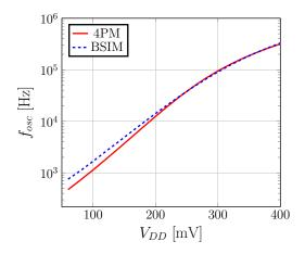
**Figure 15.** Oscillation frequency vs. the supply voltage  $V_{DD}$ .
