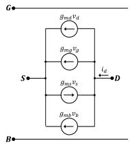
Figure 2. Low-frequency small-signal model of the MOSFET.
