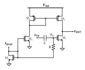
Figure 18. Common-source amplifier.
