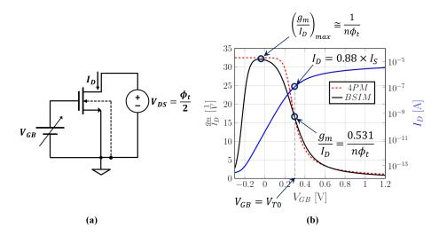
**Figure 5.** (a) Circuit to extract parameters from (b) the  $g_m/I_D$  and  $I_D$  curves.
