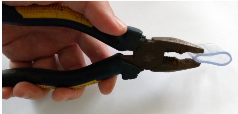
Figure 63 - Reshaping the chamber to an elliptical format.
