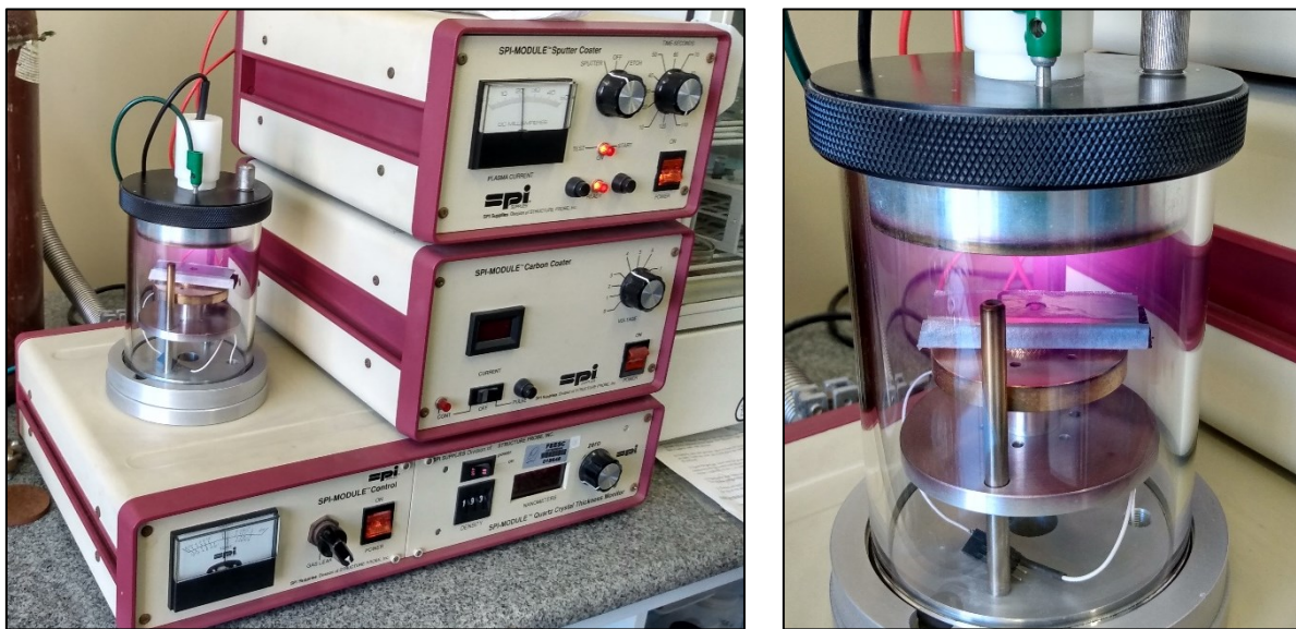
Figure 51 - (a) Sputtering process. (b) Details of the chip on the chamber.
