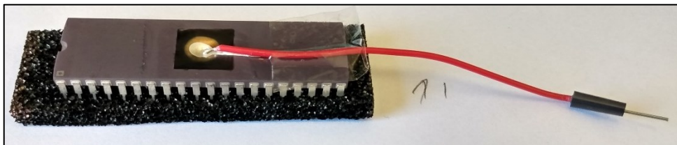
Figure 55 - Chip final assembly after metallization.
