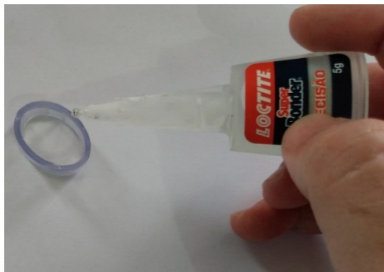
Figure 64 - Applying glue to the chamber.
